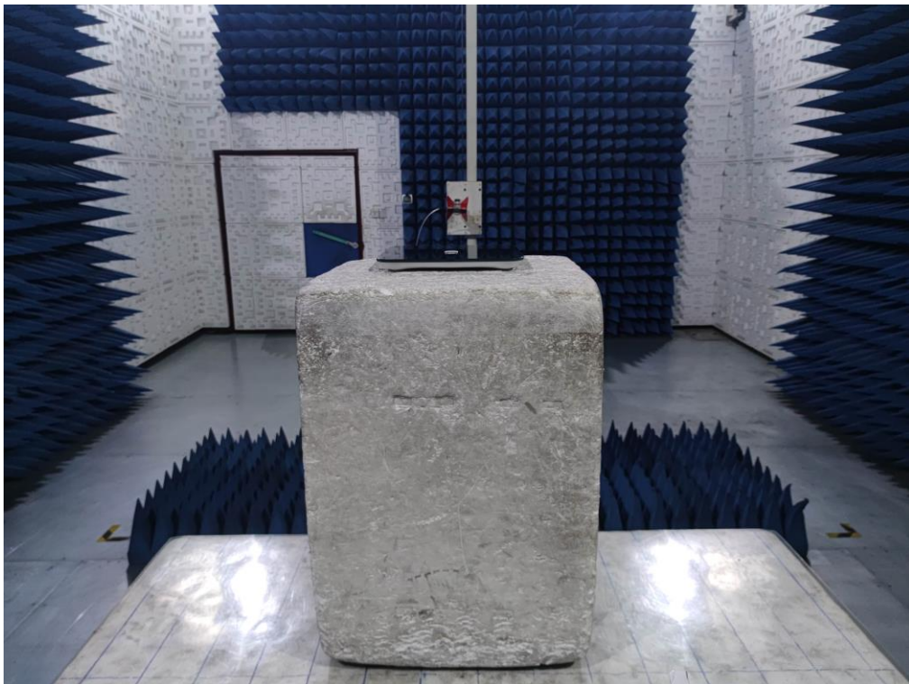
RADIATED EMISSION TEST SETUP ABOVE 1GHz
