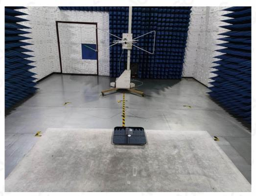
RADIATED EMISSION TEST SETUP ABOVE 1GHz
