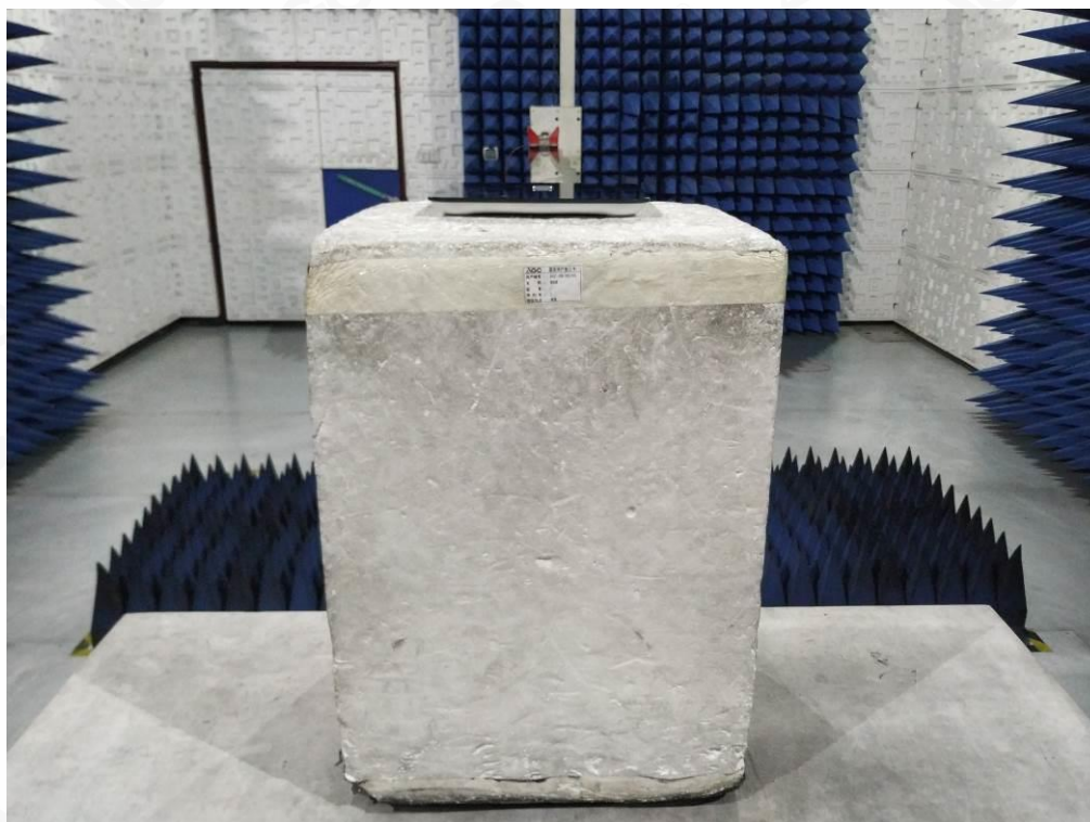
FCC RADIATED EMISSION TEST SETUP ABOVE 1GHZ
