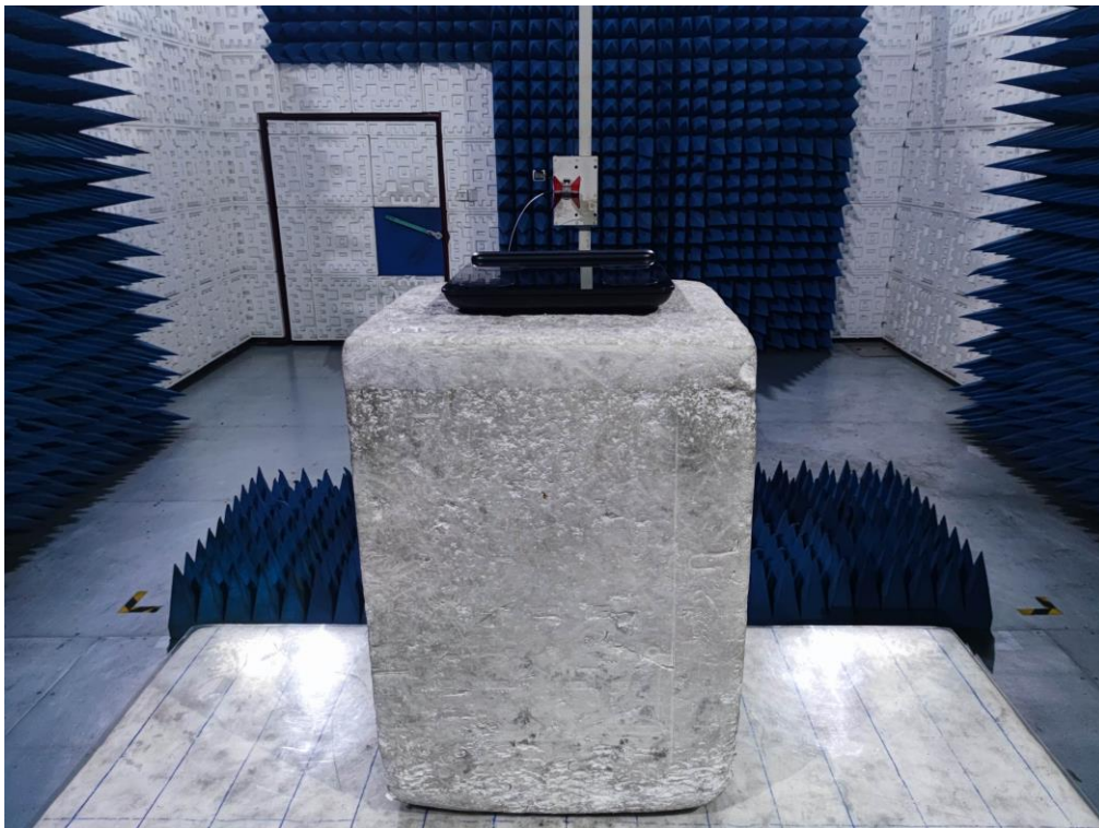
RADIATED EMISSION TEST SETUP ABOVE 1GHz
