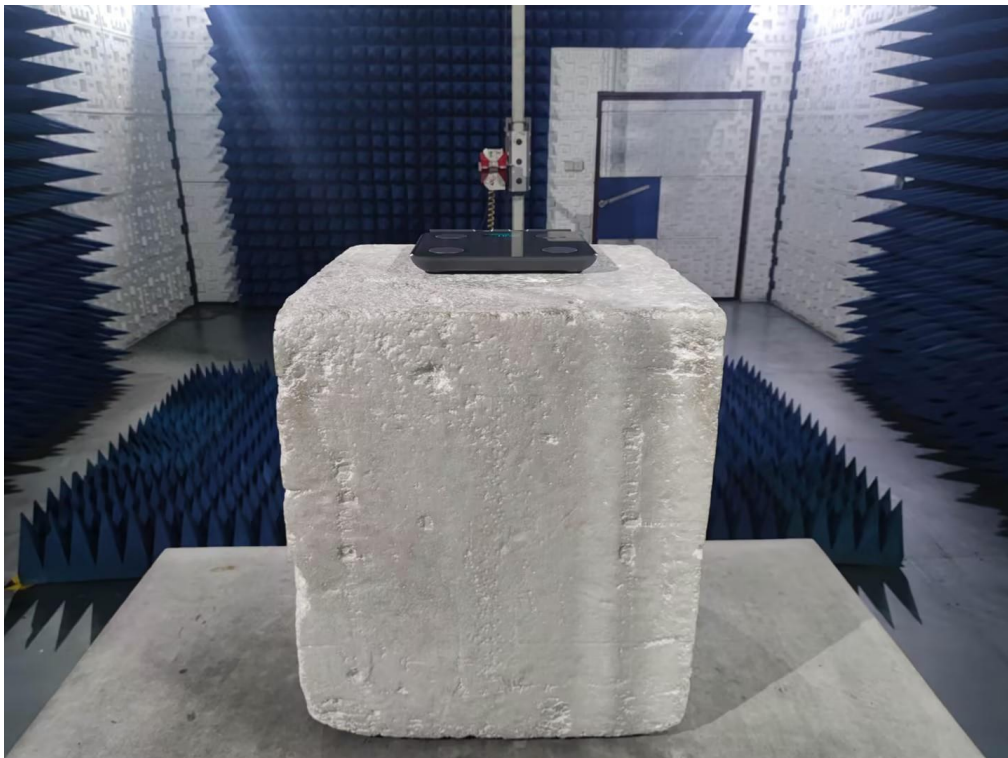
RADIATED EMISSION TEST SETUP ABOVE 1GHz
