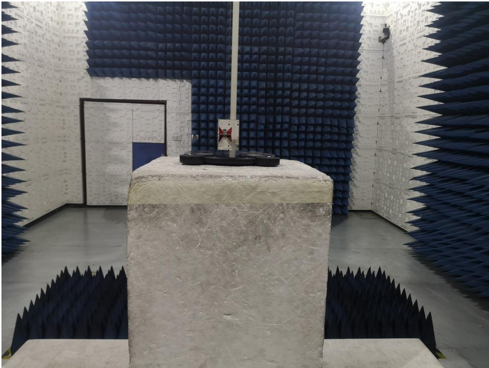
RADIATED EMISSION TEST SETUP ABOVE 1GHZ
