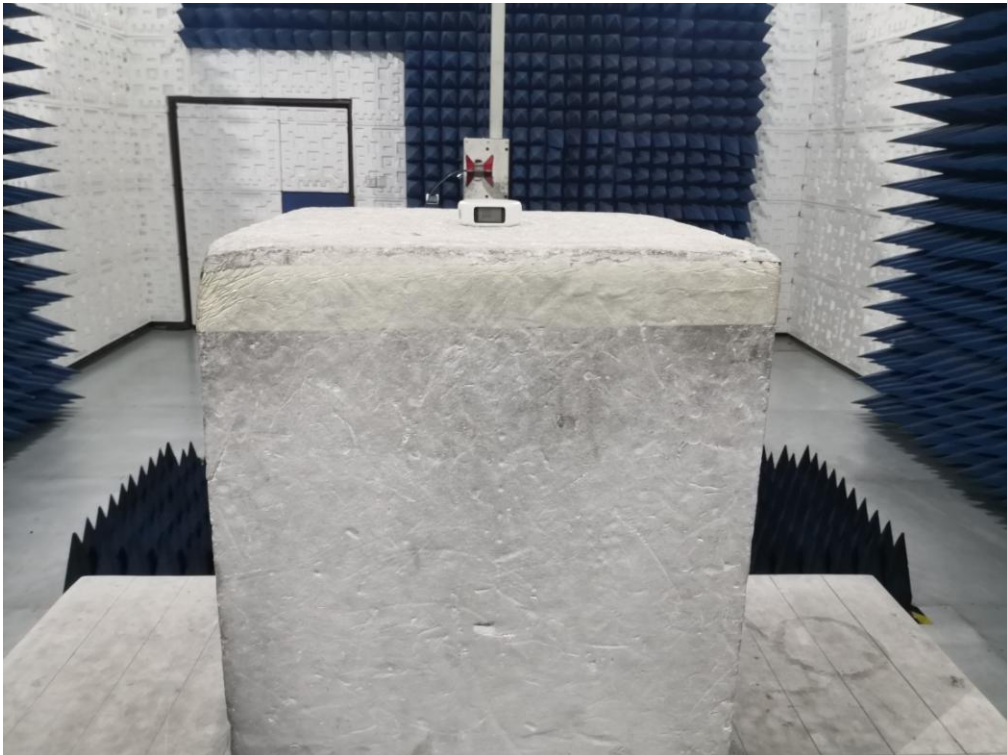
RADIATED EMISSION TEST SETUP ABOVE 1GHZ
