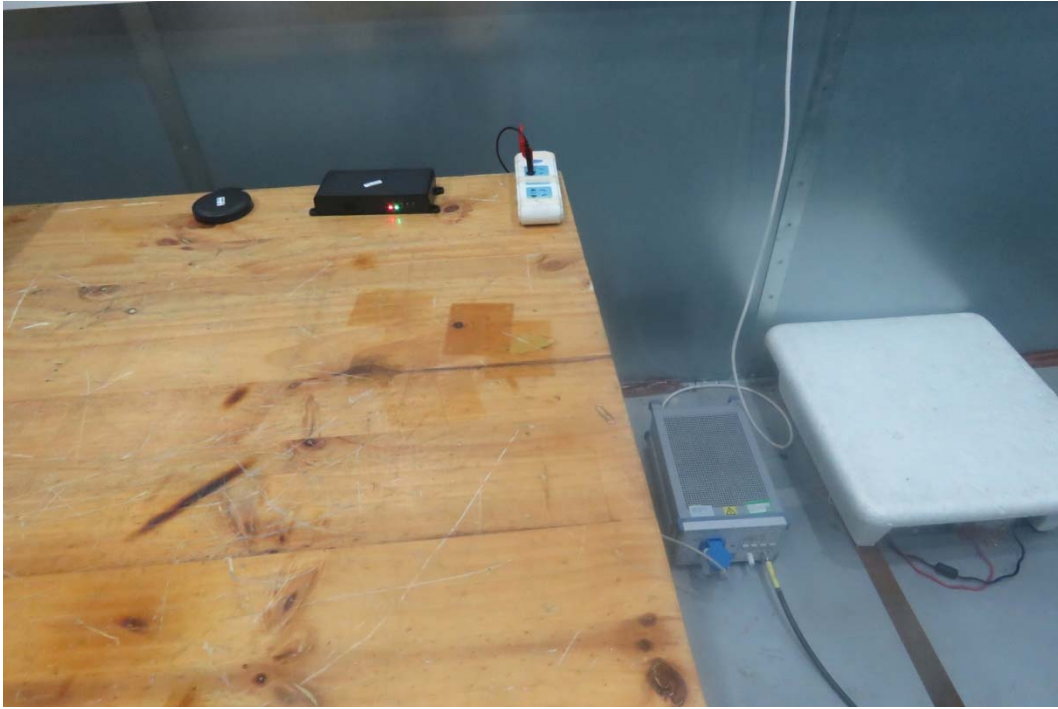
Picture 2 Conducted Emission Test Setup
