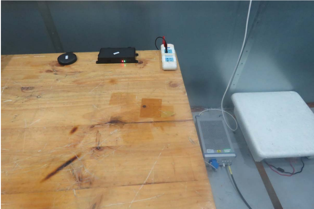
Picture 2 Conducted Emission Test Setup
