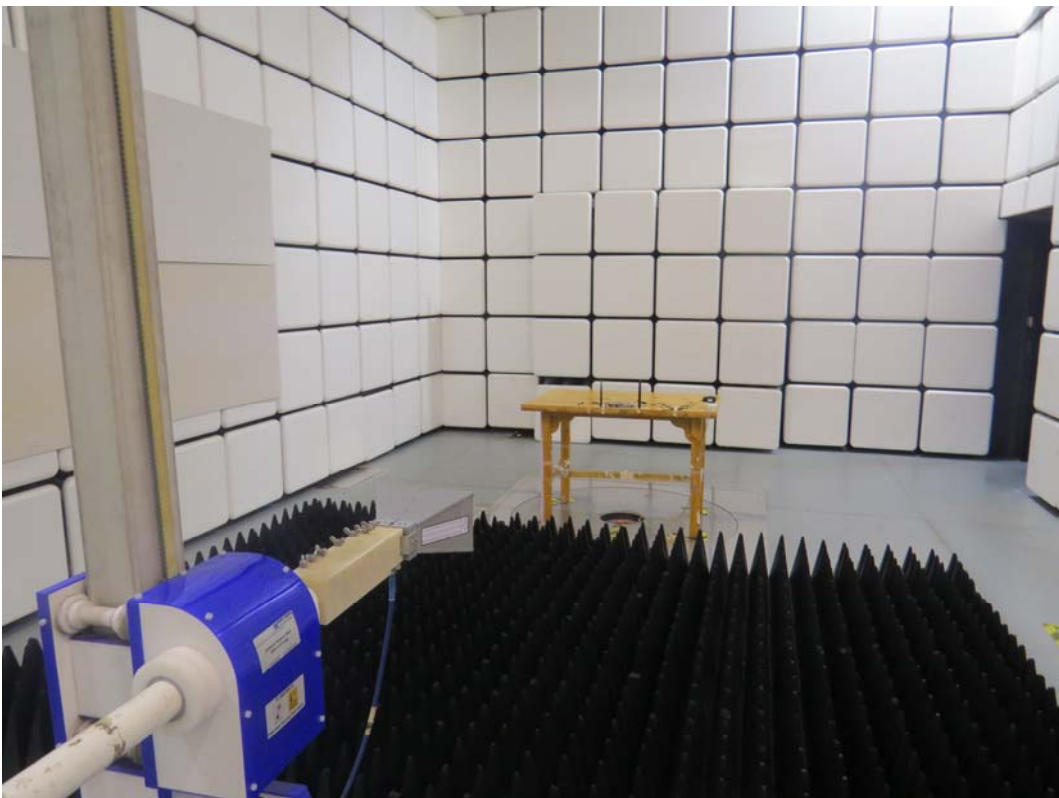
Picture 2: Radiated Spurious Emissions Test setup
