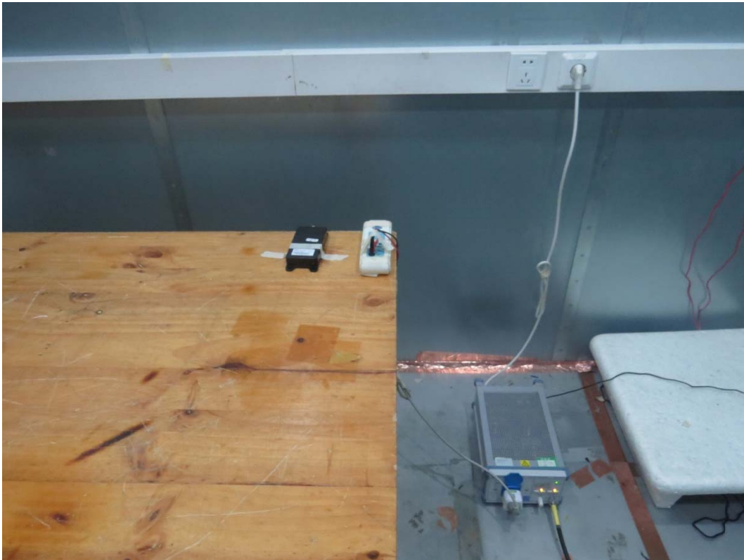
Picture 2 Conducted Emission Test Setup
