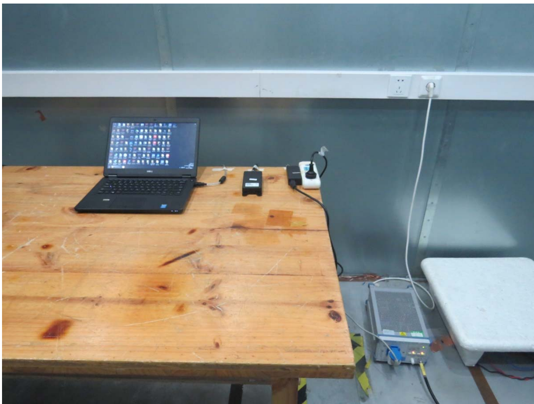
Picture 2 Conducted Emission Test Setup
