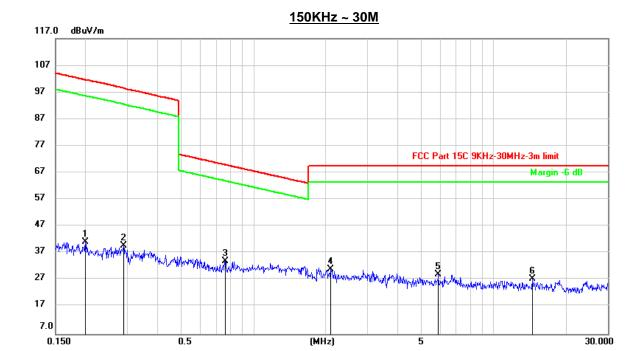
**Frequency** Reading Correct Result Limit Remark No. Margin (MHz) (dBuV) (dB/m) (dBuV/m) (dBuV/m) (dB) 0.1995 20.85 20.37 41.22 101.60 -60.38 1 peak 2 0.2878 19.66 20.31 39.97 98.49 -58.52 peak 3 0.7630 13.66 20.36 34.02 69.97 -35.95 peak 4 2.0989 10.24 20.75 30.99 69.54 -38.55 peak 5 20.87 -40.49 5.8978 8.18 29.05 69.54 peak 6 14.5168 6.50 20.94 27.44 69.54 -42.10 peak
