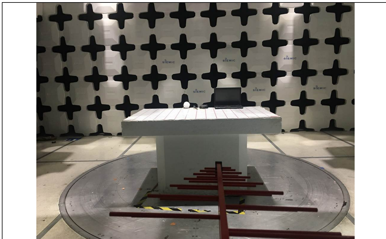
Radiated Emission Test below 1GHz Front View
