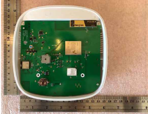
G1 PCBA bottom showing power and USB interfaces
