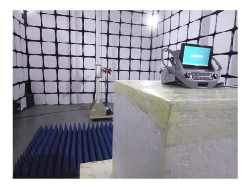
Radiation Emission Test Setup (Above 18GHz)
