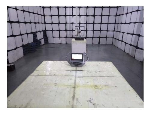
Radiation Emission Test Setup (30MHz to 1GHz)
