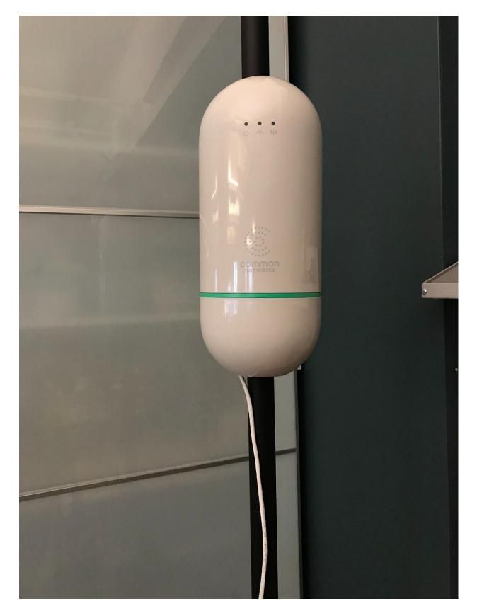
Step 8: Attached the other end of the Cat5e cable to the 54 V PoE injector. Wait while COR boots; COR will be ready when the power LED is solid green.
