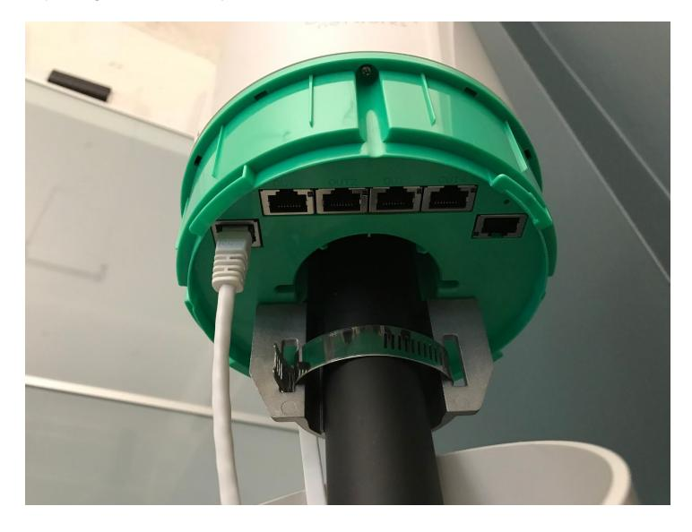
Step 7: Reattach bottom white plastic cover by sliding it into place and rotating (clockwise from below)
