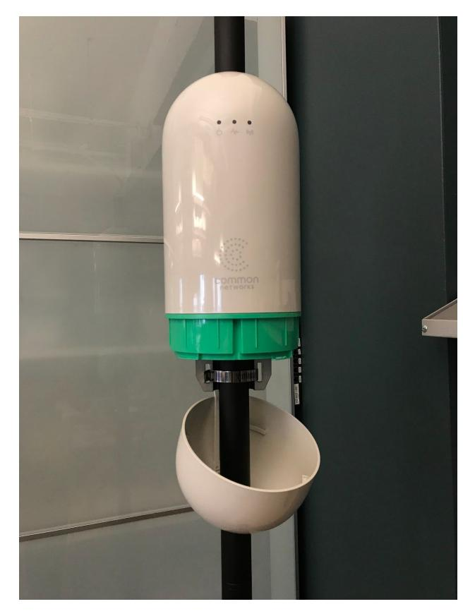
Step 4: Slide hose clamp through mounting bracket and tighten with an 8 mm socket wrench
