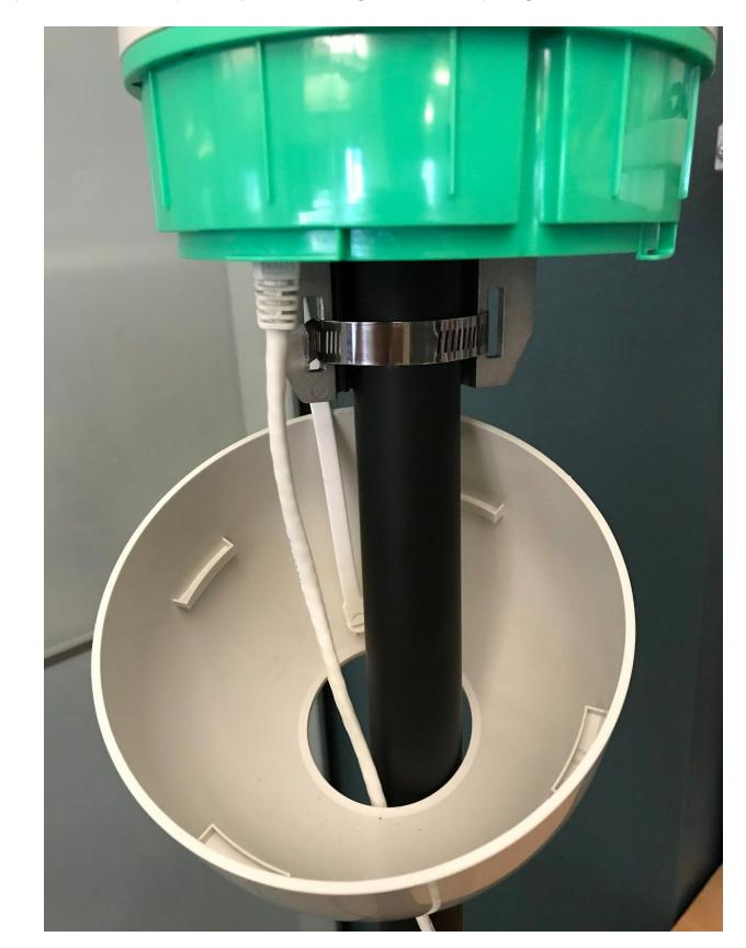
Step 5: Pass the Cat5e power input cable through the circular opening in the bottom cover
