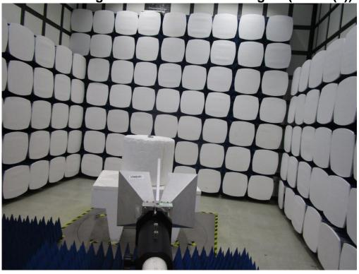
1.2 Radiated Emissions Test Setup
