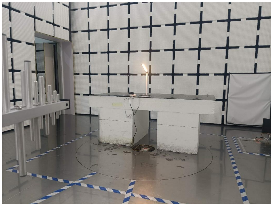
Radiation Emission View (30MHz to 1GHz)
