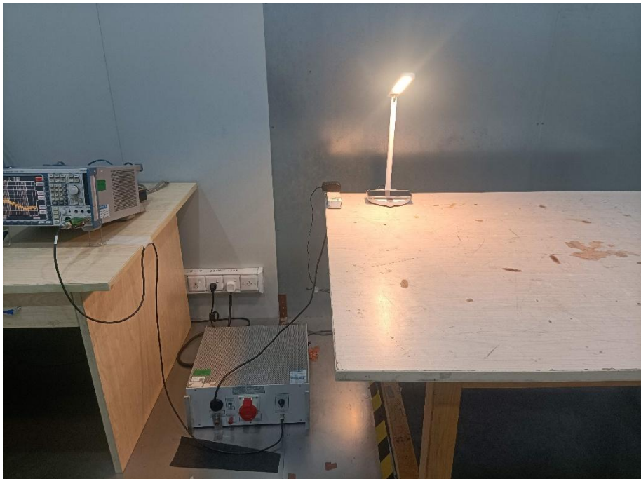
Conducted Emission Test Setup
