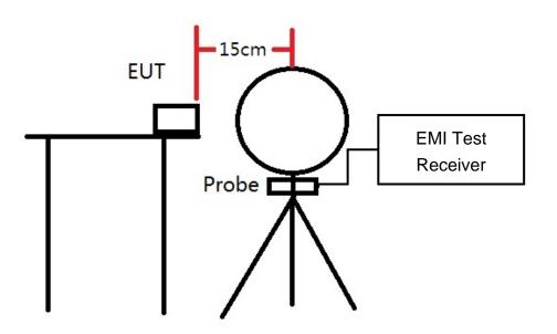
These testing were performed at test configuration as above diagram.
