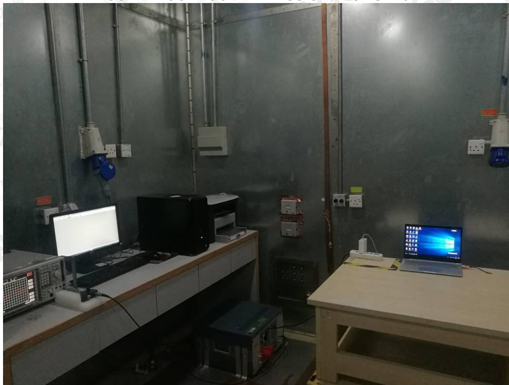
FCC RADIATED EMISSION TEST SETUP
