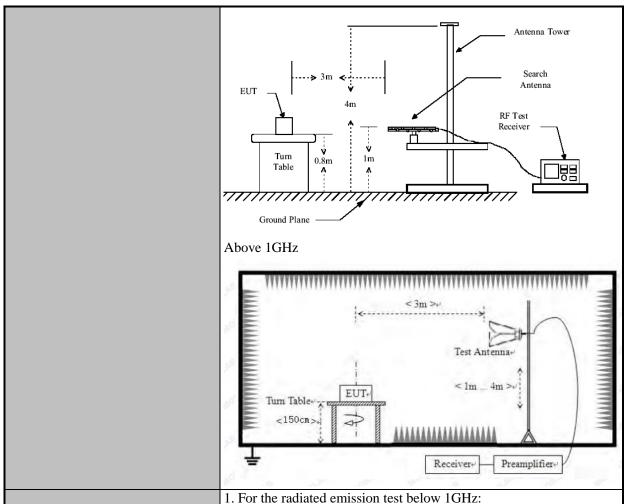
The EUT was placed on a turntable with 0.8 meter above ground. The EUT was set 3 meters from the interference receiving antenna, which was mounted on the top of a variable height antenna tower. The EUT was arranged to its worst case and then tune the antenna tower (from 1 m to 4 m) and turntable (from 0 degree to 360 degrees) to find the maximum reading. A pre-amp and a high PASS filter are used for the test in order to get better signal level.
