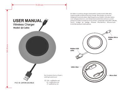
Specification: Input: QC2.0&3.0 Adapter 5V/3A 9V/2A Output: SV/1A Wireless Output: DC5V/1A; DC9V/1.1A
