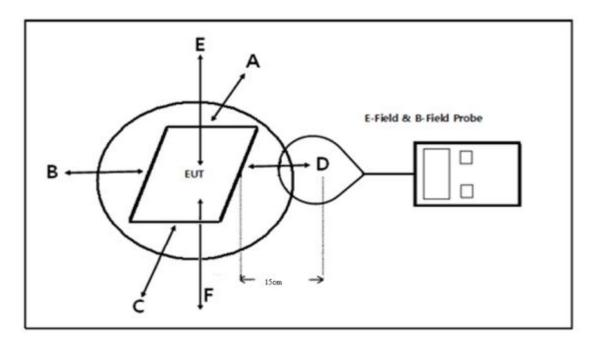
For mobile RF exposure condition, due to installation limitations no tests from the underside of the charging device are required.
