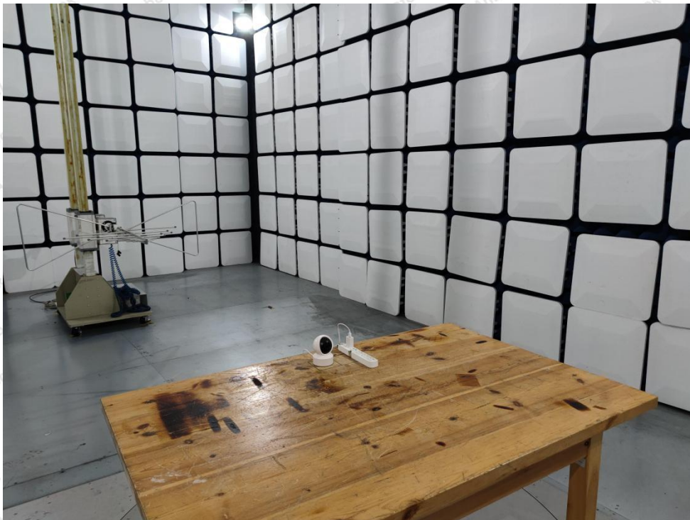
Photo of Radiation Emission Test
