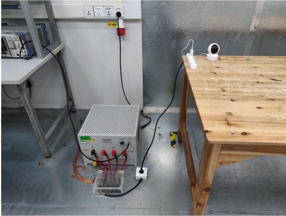
Photo of Power Line Conducted Emission Test
