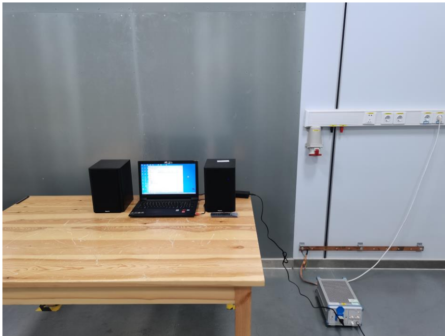
Fig. 4 Power line conducted emission setup photo
