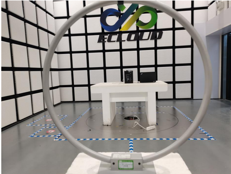
Fig. 1 Radiated emission setup photo(Below 30MHz)
