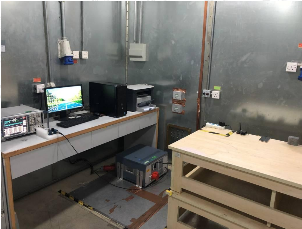
FCC RADIATED EMISSION TEST SETUP
