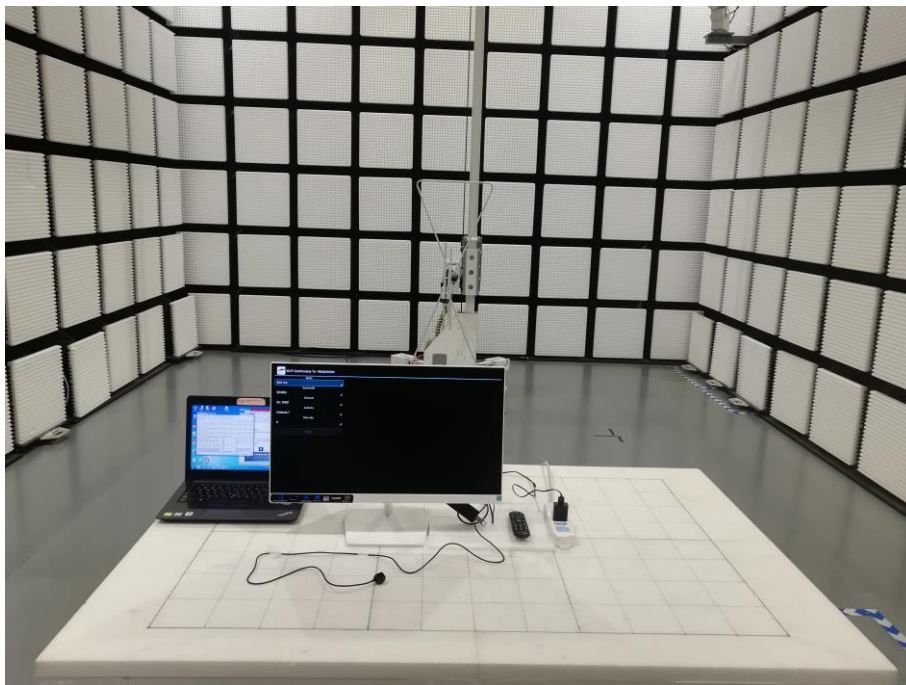
Fig. 2 Radiated emission setup photo(30MHz-1GHz)
