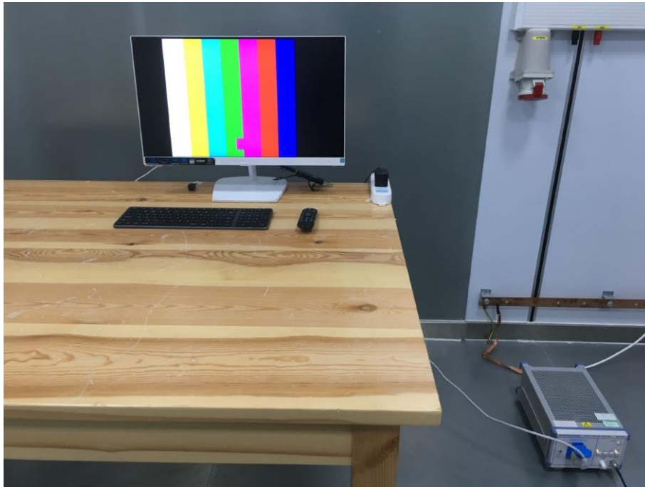
Fig. 4 Power line conducted emission setup photo
