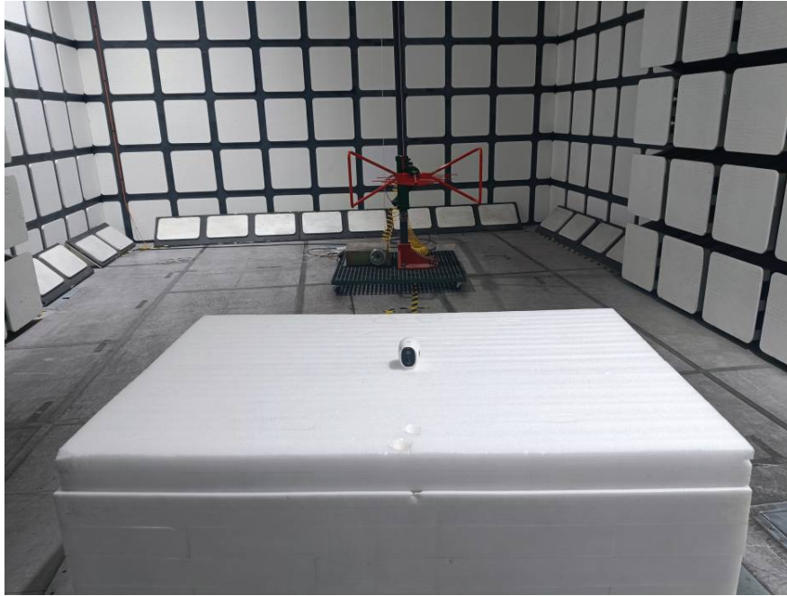
Radiated Spurious Emissions View (Below 1 GHz)
