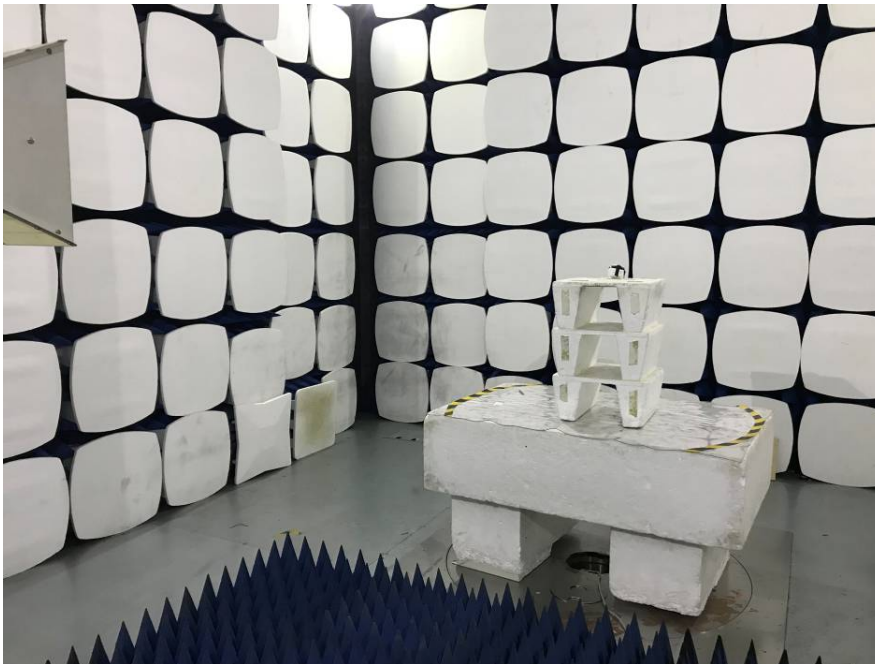
Radiated Spurious Emissions View (Above 1 GHz)
