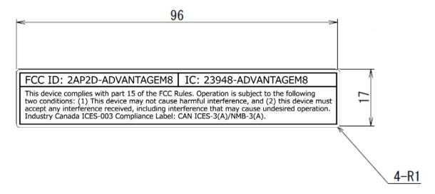
The Label is permanently affixed on the device with an adhesive.
