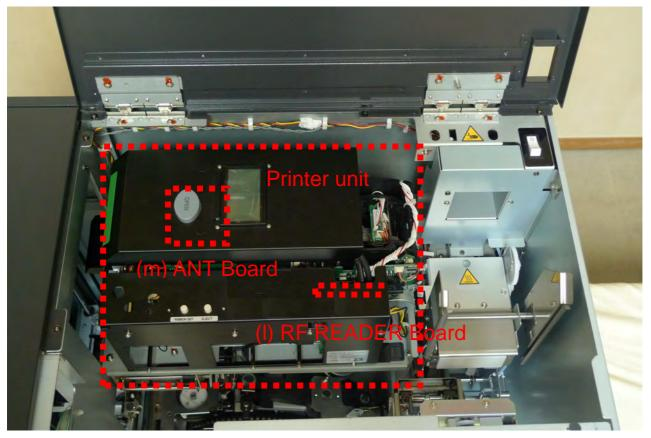
• The locations of "(1) RF READER Board" and "(m) ANT Board" - View with open the right cover
