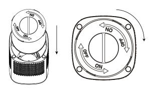
3). Put the filter into the machine and turn it clockwise to the buckle. After the filter is rotated in place, you will hear a squeak (as shown in the right picture).
