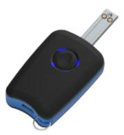
ZMK3-1U Smart Electronic Key built-in financial level security chip, unable to copy and crack. Built in rechargeable lithium battery provides power for intelligent lock core. After receiving the encryption command, the smart key is encrypted and authenticated with the lock core. After the authentication is passed, the intelligent lock core can be opened.
