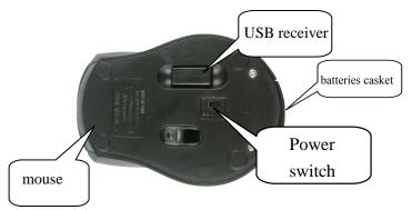
b. Put the batteries into the batteries casket, lock the cover.
