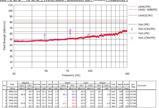
Test mode : 3 GHz ~ 18 GHz (Worst case : Bluetooth LE / Middle Frequency)
