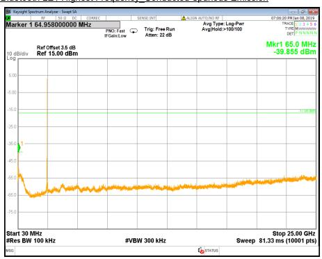
Test mode : Bluetooth LE / Highest Frequency\_Conducted Spurious Emission
