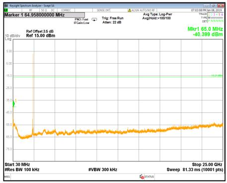
Test mode : Bluetooth LE / Lowest Frequency Conducted Spurious Emission
