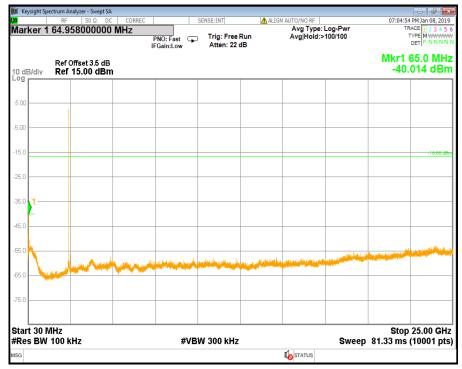
Test mode : Bluetooth LE / Middle Frequency Conducted Spurious Emission
