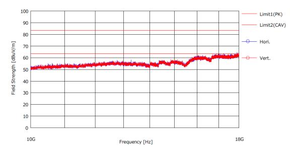
$\begin{array}{lll} \mbox{Note 1:} & \mbox{Measured distance: 1 m} \\ \mbox{Note 2:} & \mbox{Limit: Peak: 83.5 dB} \mu\mbox{V/m} \\ & \mbox{Average: 63.5 dB} \mu\mbox{V/m} \\ \end{array}$
