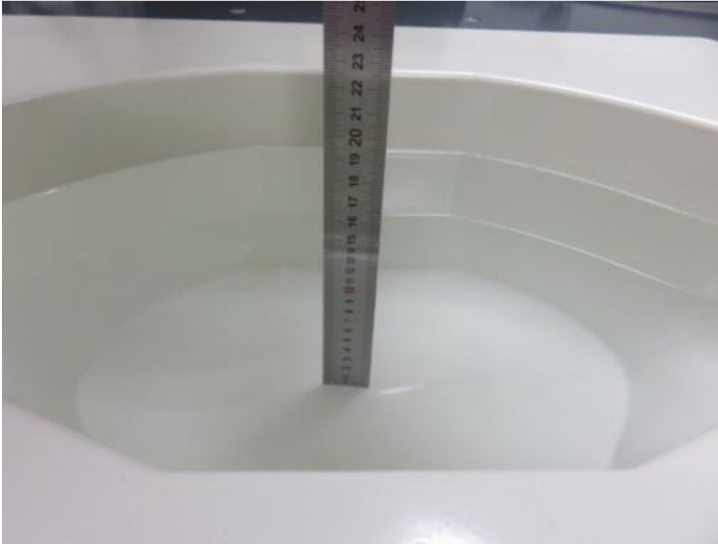
Photograph of the depth in the Body Phantom (835MHz, 15.4cm depth)
