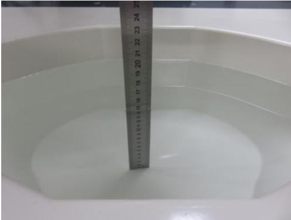
Photograph of the depth in the Body Phantom (2450MHz, 15.2cm depth)
