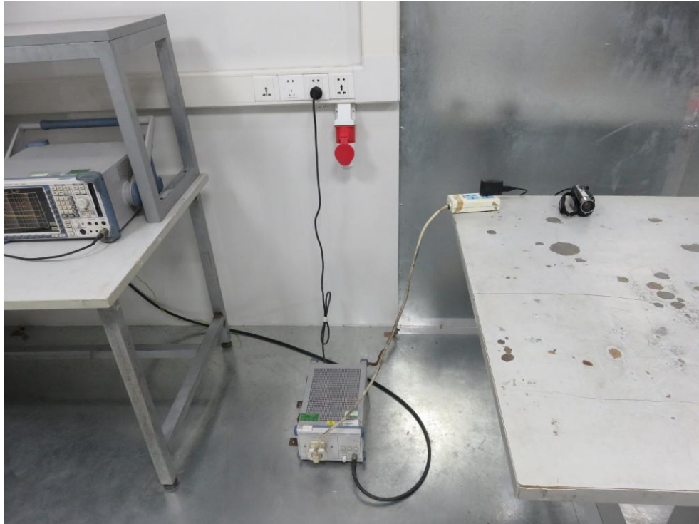
Photo of Radiation Emission Test
