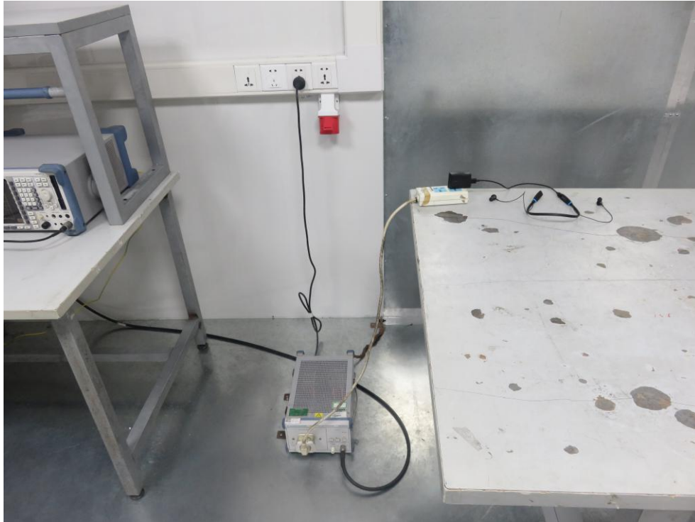
Photo of Conducted Emission Measurement
