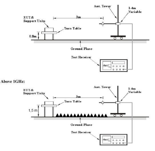
The radiated emission Below 1GHz tests were performed in the 3 meters chamber A, above 1GHz tests were performed in the 3 meters chamber B, using the setup accordance with the ANSI C63.10-2013. The specification used was the FCC 15.209, and FCC 15.247 limits.
