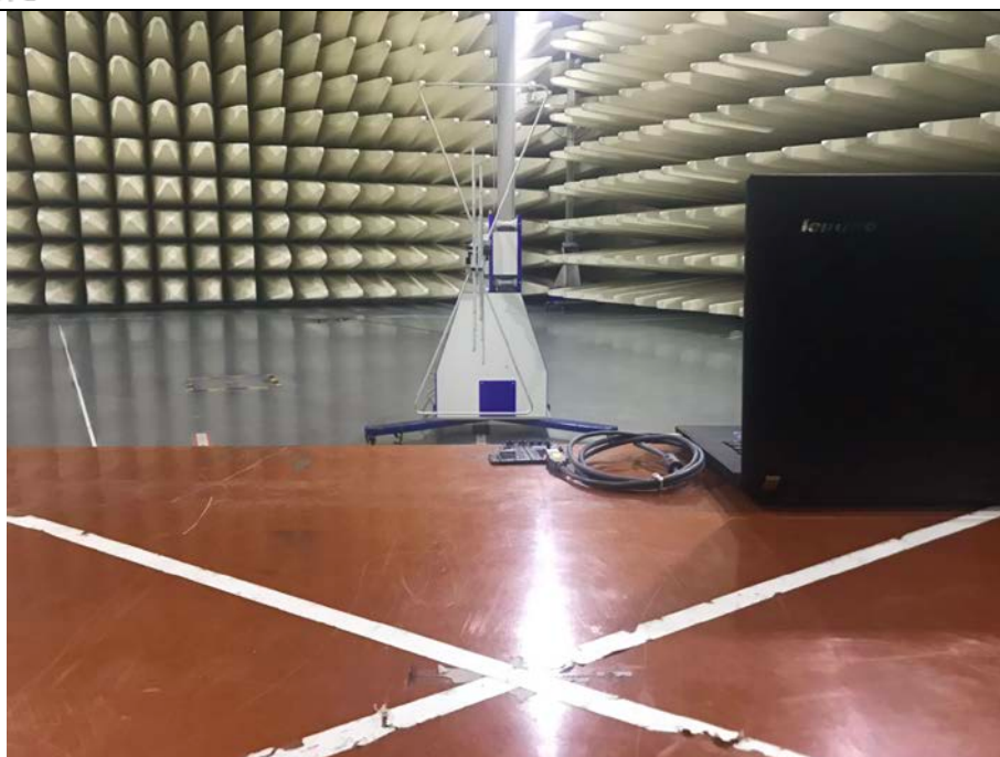
Spurious Radiated Emissions Test setup
