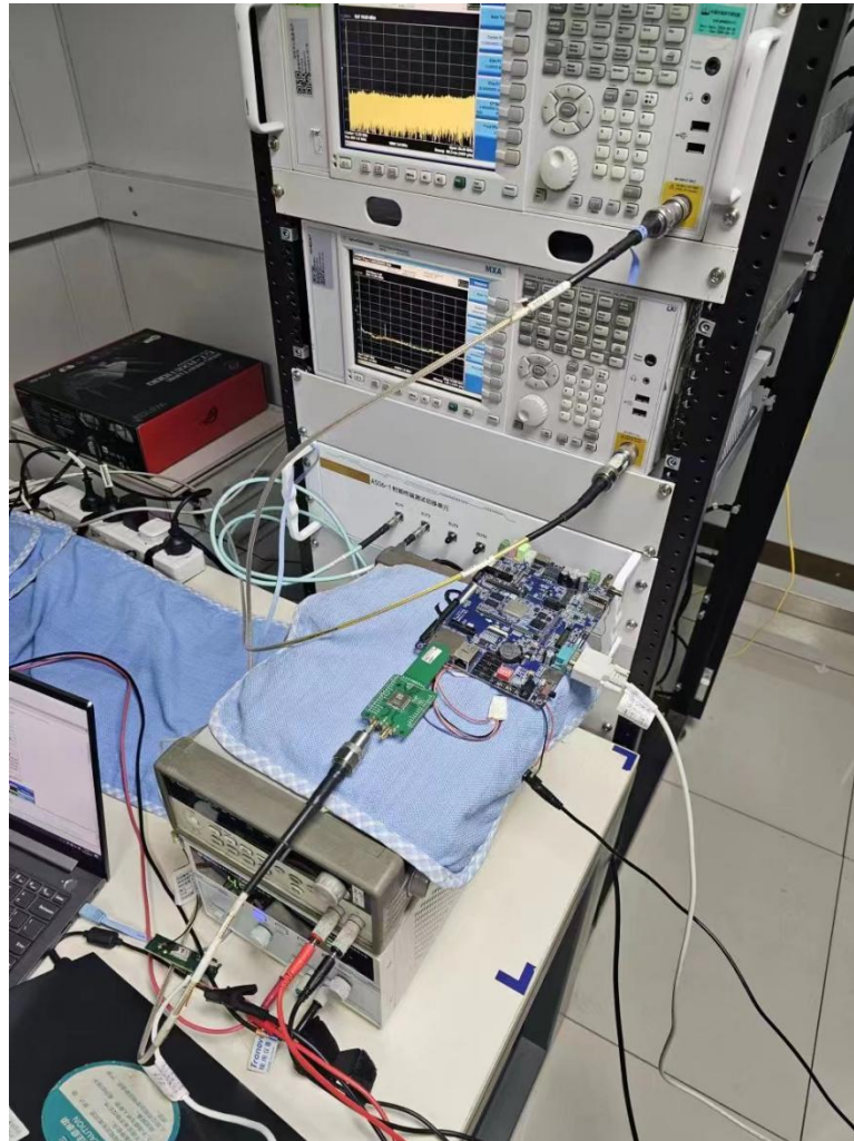
RF Conducted Test setup (BT/WIFI)
