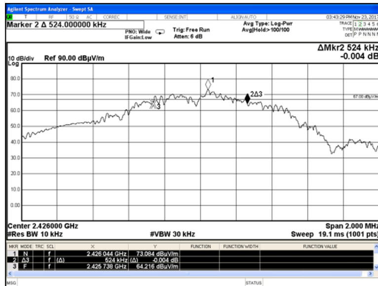
Plot 7.1.2 The 6 dB bandwidth test result at mid frequency
