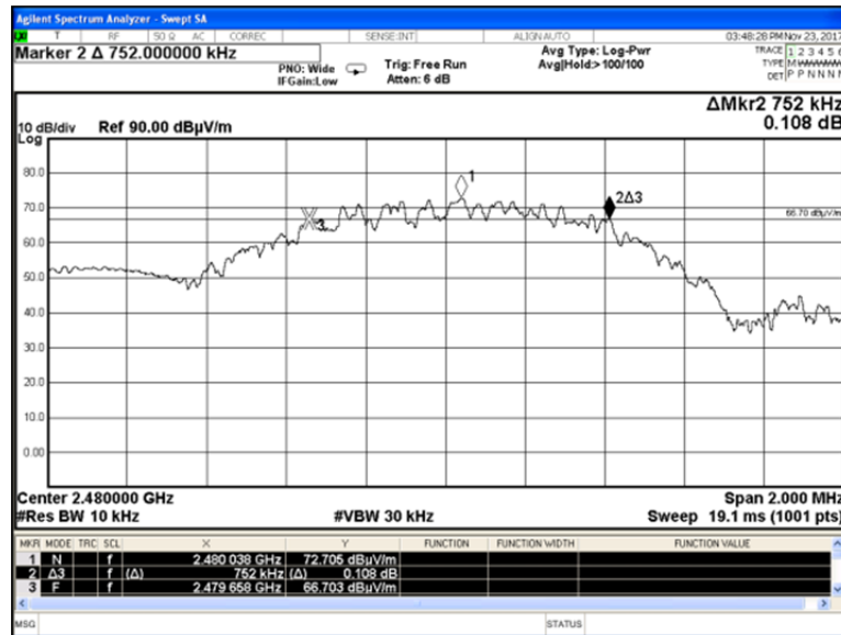
Plot 7.1.3 The 6 dB bandwidth test result at high frequency
