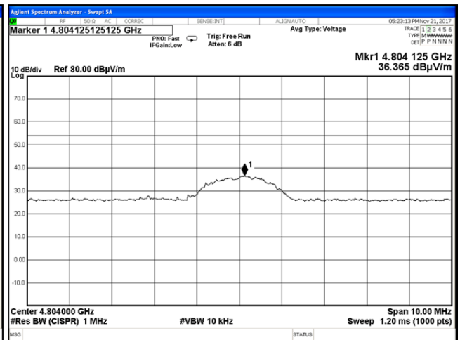
Plot 7.3.24 Radiated emission measurements at the second harmonic of low carrier frequency
