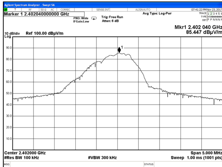
Plot 7.4.1 The highest emission level within the assigned band at low carrier frequency
