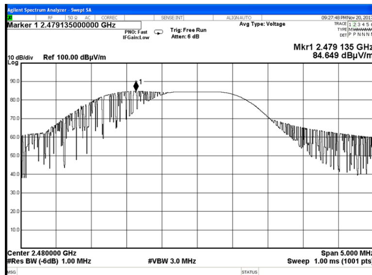
Plot 7.2.6 Field strength of carrier at high frequency in horizontal antenna polarization
