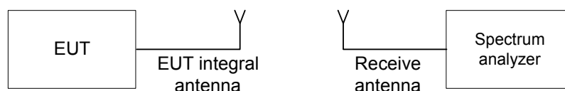
Figure 7.1.1 Setup for transmitter shut down test
