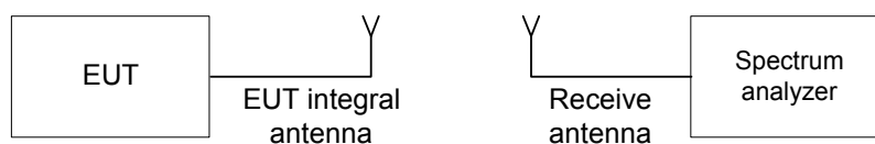
Figure 7.1.1 Setup for transmitter shut down test
