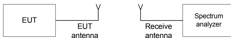
Figure 7.3.1 Occupied bandwidth test setup
