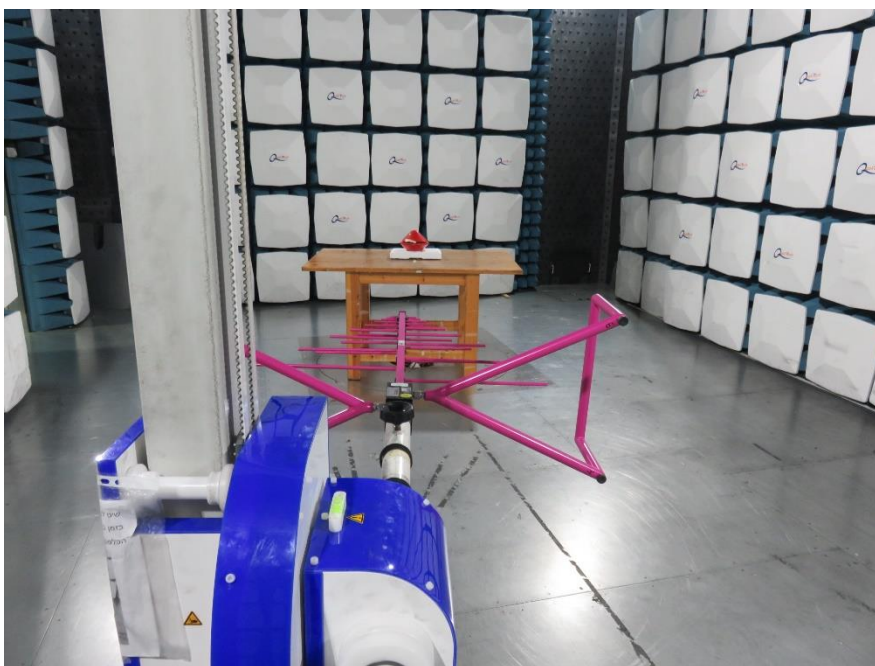
Photograph 2: Radiated Emission Testing
