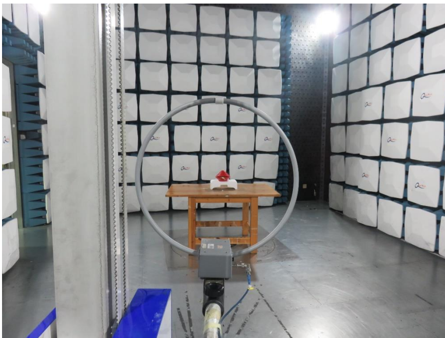
Photograph 2: Radiated Emission Testing
