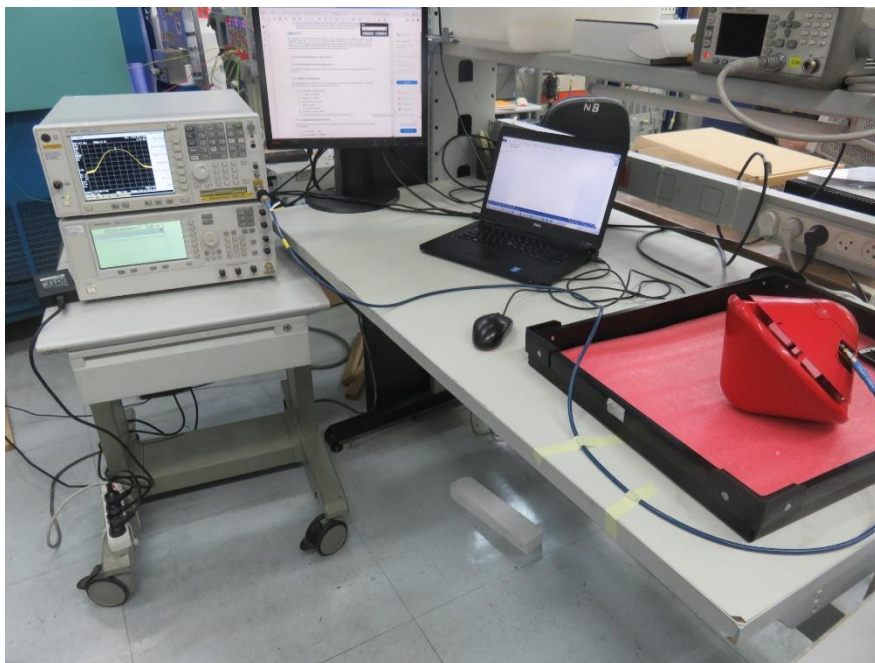
Photograph 4: Conducted Emission Testing
