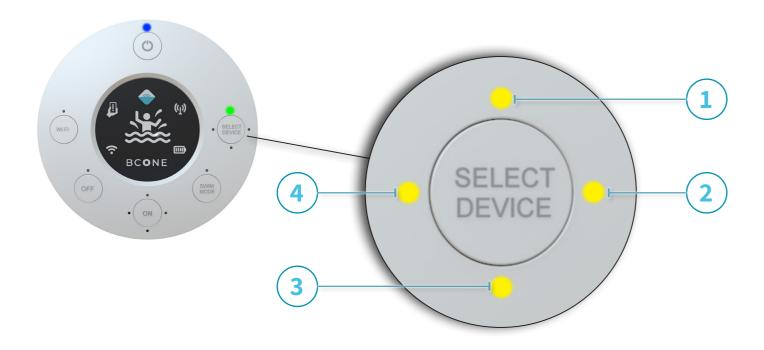
After selecting a Pool Unit, one of the operation mode LEDs lights up for a few seconds to indicate the current operation mode.
