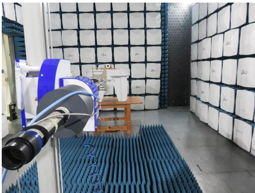
Photograph 3: Radiated Emission Testing 1GHz-18GHz
