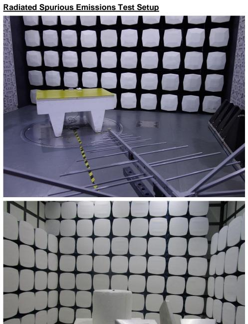
Radiated Emissions which fall in the restricted bands Test Setup
